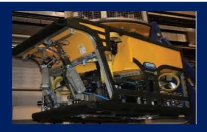
Quasar is the medium size vehicle in SMD's Q-Series Work ROV range. Utilising the latest "multi-platform" Curvetech components, the vehicle offers class leading performance and exceptional tooling capability.
