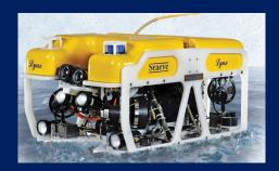
The Seaeye Lynx are widely regarded as the leading inspection class vehicle within the oil and gas industry. Increasingly they are also being taken up as the ROV of choice by military and scientific customers seeking increased capabilities in deep water. With a depth rating of 1500m, the Lynx has a very stable platform and is able to perform well in strong currents and under the harshest conditions, providing excellent handling and maneuverability.
